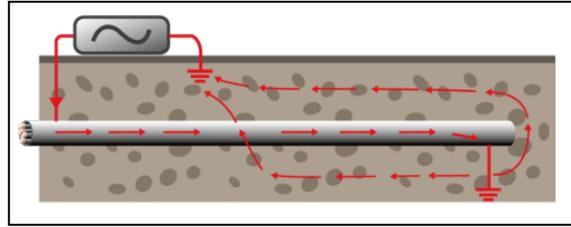
One of the main reasons that utility locators cannot locate previously installed trace wires is because they improperly terminate without going to ground. For example, at a hydrant or in a valve box or manhole, if the trace wire is not properly grounded, the AC current will not follow the trace wire, and will not have a return path back to the transmitter. A complete circuit does not exist; thus, a locatable signal cannot exist.
